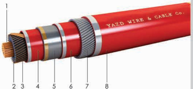
XLPE insulated single core lead sheathed armoured 6kv up to 230kv
